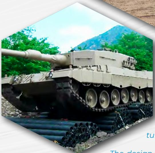
*The Chilean Army asked FAMAE to modify a Leopard 1V tank to enable it to transport and launch tube bundles to overcome obstacles in the field. This version of an armored engineering vehicle consists of an armored dome to cover the crew compartment, a rear and a front tilting platform, designed to transport three heavy tube bundles and launch them into deep trenches.*
